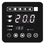
After completing the defrosting, the unit will be automatically switched to the heating/automatic mode (keeping consistent with the mode before defrosting).
